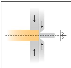
The centering jaws and the blades are programmable for each layer, independently of each other. The blades cut linearly and perpendicularly to the cable axis and are arranged adjacent to the centering jaws.
